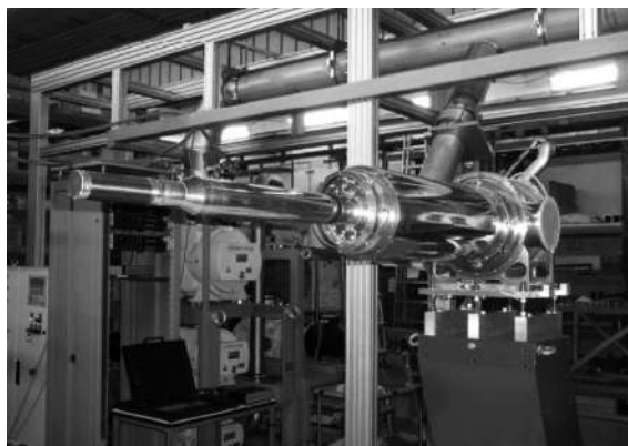
Fig. 6. The dilution refrigerator with longitudinal holding coil
